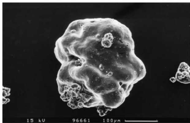
Figure 4. Scanning electron micrograph of a shellac-coated pectin amide/maltodextrin capsule (system 3, SL).
